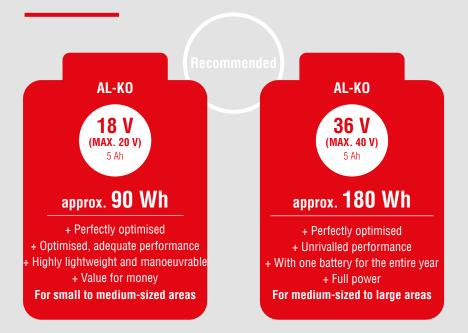
The nominal voltage (18 V / 36 V) is the voltage in normal operation. The maximum voltage (max. 20 V / 40 V) indicates the maximum measurable value reached at the end of charging.
